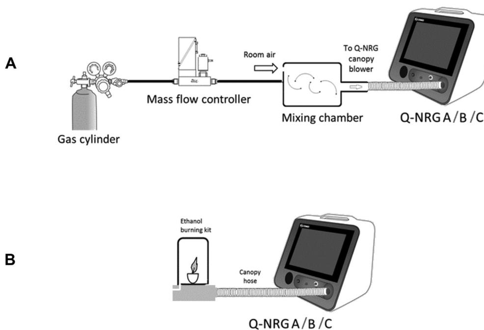
Fig. 2. *In vitro* setup for canopy dilution (A) and ethanol burning tests (B).
