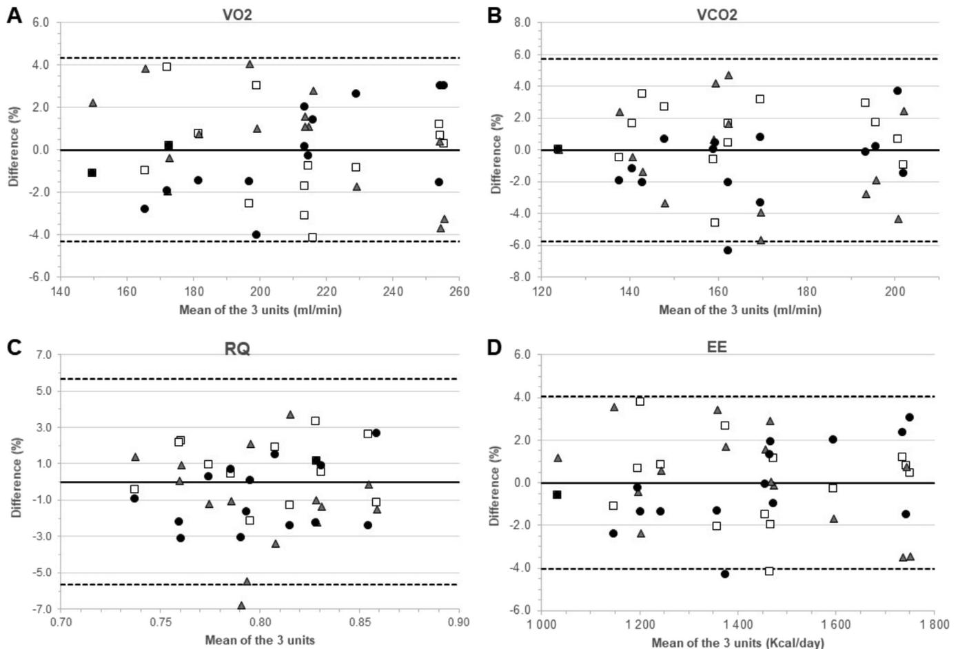
**Fig. 4.** Adjusted Bland-Altman plots for VO<sub>2</sub>, VCO<sub>2</sub>, RQ and EE. The three Q-NRG® units are shown in different shapes (unit A = white square, unit B = grey triangle, unit C = black circle).
