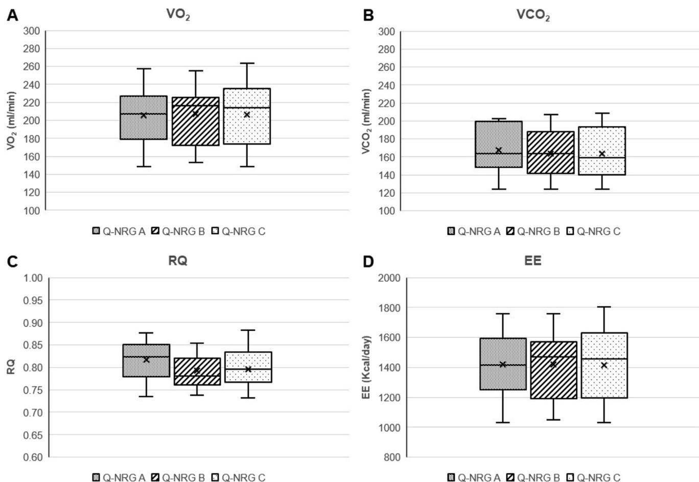
Fig. 3. Box plots showing VO<sub>2</sub>, VCO<sub>2</sub>, RQ and EE values obtained *in vivo* by each of the three Q-NRG® units (unit A = grey, unit B = stripes, unit C = points).
